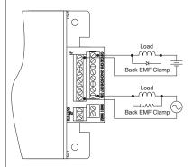
Wiring Recommendations for relay outputs
